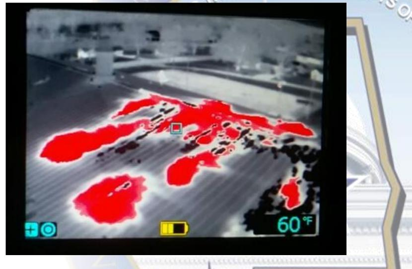
Thermal imaging of the roof system caused concerns about possible collapse of the roof system. The fire department would not risk putting personnel on the roof.
